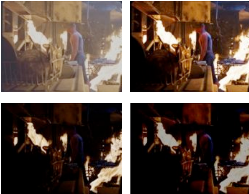
An original log film plate (top-left) is loaded into the DI color corrector. When viewed with a film emulation table (top-right), the appearance is predictive of the final output with a default exposure. If we were to lower the exposure using an additive offset in log-space (lower-left), new details in the flame highlights are revealed. When a similar correction is applied to a color-corrector working in a display-referred space (lower-right), this detail is lost. Imagery from “Spider-Man” Courtesy of Columbia Pictures. © 2002 Columbia Pictures Industries, Inc. All rights reserved.
